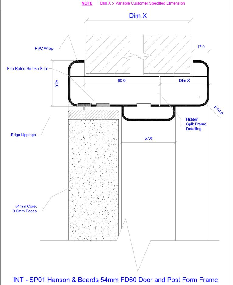
INT - SP01 Hanson & Beards 54mm FD60 Door and Post Form Frame Vertical Through Sectional Drawing Detail
